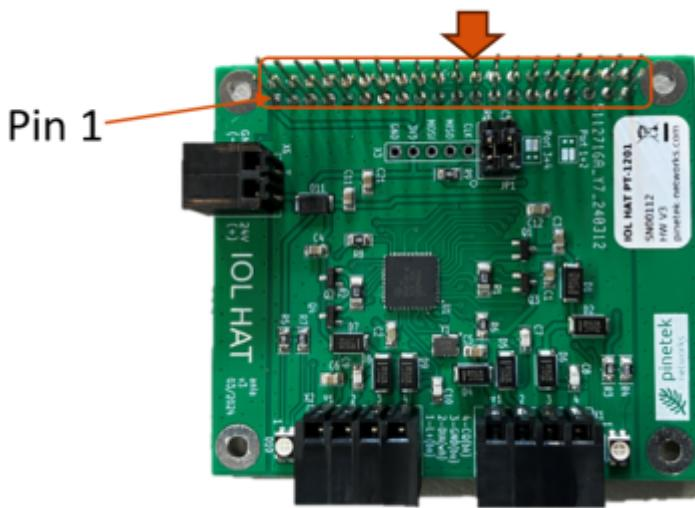
This connector is implemented as stack-through, i.e. up to two IOL HATs can be connected on top of each other. If the pins are not occupied by the connected IOL HAT, additional expansion boards can be connected via the stack-through connector.
