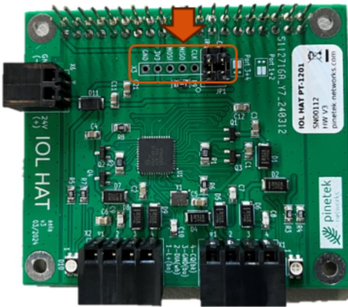
The 40-pin connector is not populated, the X3 connector is populated with the pin header. Selection over the jumpers is not possible. The interface to the host system is on X3 with the following pin assignments:
