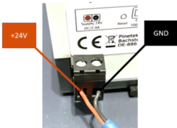
The Pinebox operates on 24V DC with a max. deviation for +/- 20% (i.e. 20,2V-26,8V). At maximum load, the device has a current consumption of 2,8A (at nominal voltage of 24V). The user shall ensure that the limits for safe operation of the device are maintained at power input.
